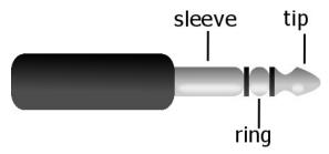
The exp jack is connected to the pedal like this: sleeve : ground ring: 3.3V supply voltage tip: controlling (varying) pin
