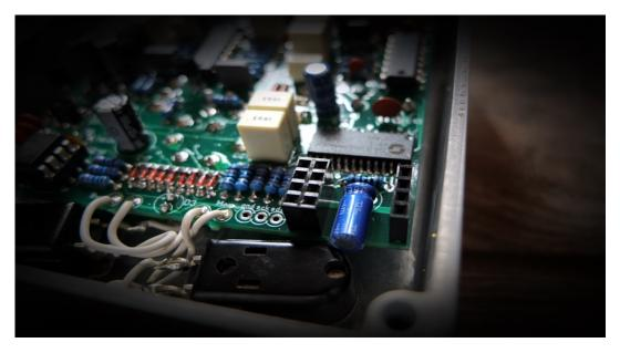
Inside your pedal you will find the socket for the molecular module on the bottom right side of the circuit board:
