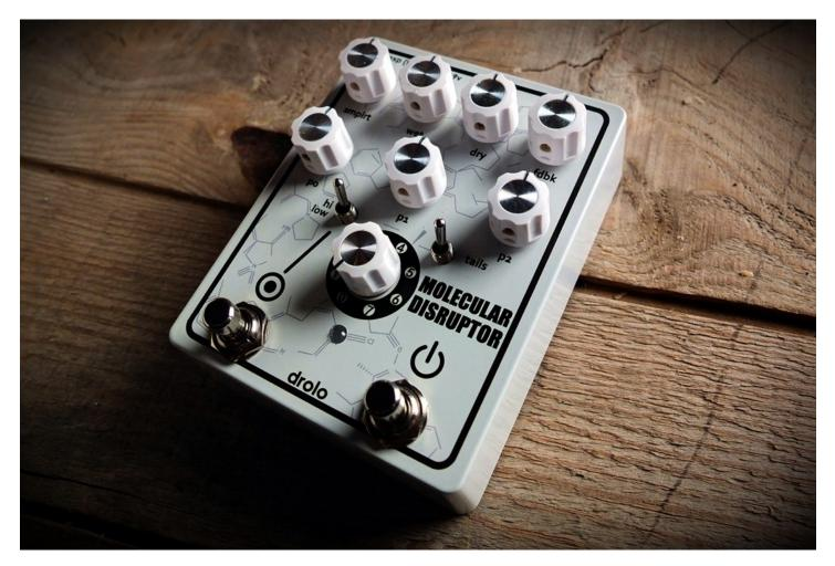
The Molecular Disruptor is a DSP based multi-effect pedal that can be loaded with 8 patches selected from the molecular patches list: <u>http://www.davidrolo.com/molecular-patches/</u> This list is regularly being updated with new patches.
