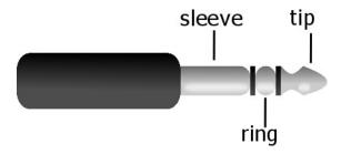
The exp jack is connected to the pedal like this:
